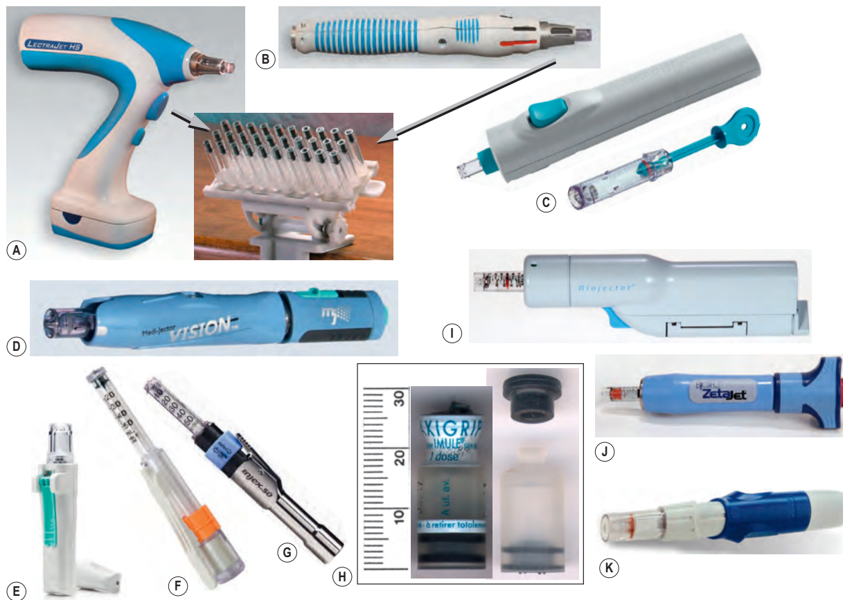
Figure 61-6 Selected Disposable-Syringe Jet Injectors (DSJIs), Licensed or Investigational (as noted). (A) Investigational LectraJet HS (high-speed) motorized DSJI (D'Antonio Consultants International 613 ) features built-in motor and rechargeable battery for rapidly compressing metal spring between injections at rates exceeding 600 per hour, with battery capacity of > 3,000 injections per charge. Capable of rapid, fingers-free loading and unloading of single-use syringes from (A, inset) a sterile-packaged, 30-unit magazine for mass vaccination. Magazine may also be mounted on nondominant forearm for vaccinator mobility. Capable of backup manual spring-cocking if batteries are depleted. (B) LectraJet M3 (manual) model DSJI, 613 sharing the same common syringe as the adjacent HS model for rapid, fingers-free loading and unloading of syringes. IM or SC delivery set by varying syringe orifice diameter. Cocked using off-tool carrying case (not shown). Cleared for US marketing by FDA in 2009. Syringes and needle-free vial adaptors also supplied in individually wrapped sterile envelopes for routine immunization (not shown). (C) PharmaJet Stratis 62 DSJI, for 0.5-mL dose delivery. Delivery IM or SC set by vaccinator technique (fat layer pinched up for SC). Cocked using off-tool carrying case (not shown). (C, inset) Syringe is filled by pulling back and breaking off its blue shaft and thumb tab from conventional single-dose and multidose vials using needle-free vial adaptor (not shown). On insertion into device, any excess liquid is returned to vial to minimize wastage of overflow. Cleared for US marketing by the FDA in 2011. See Figure 61-2J for intradermal DSJI from same device manufacturer. (D) Medi-Jector Vision DSJI, 731 used primarily for self-administration by patients of insulin and other medications. (E) Sumavel DosePro single-use DSJI (Zogenix 734 ), licensed as drug-device combination product for subcutaneous delivery of prefilled sumatriptan for treatment of migraine and cluster headaches. 735 Uses novel, borosilicate-glass dose chamber prefilled by drug manufacturer. (F) J-Tip, single-use DSJI, 733 powered by compressed nitrogen gas. (G) Injex DSJI, 732 metal spring compressed by separate cocking device. (H) Imule manufacturer-prefilled DSJI syringe 660,737 for Vaxigrip influenza vaccine (Institut Mérieux/Pasteur Mérieux Sérums & Vaccins 736 ). The syringe served as both primary vaccine packaging in a presentation smaller than conventional single-dose glass vial (millimeter scale on left), as well as the single-use disposable syringe for jet injection. Upon removing the label (H, center), inserting into the Mini-Imojet DSJI (not shown), and removing the rubber cap (H, right), the dose was ready for injection. Studied in human trials for five vaccines 134,648,650 and found successful in immune responses and safety. Subsequently abandoned by the manufacturer. (I) Biojector 2000 DSJI (Bioject Medical Technologies 83 ), capable of subcutaneous and intramuscular injections using syringes of differing orifice diameters. 614 Cleared for US marketing by FDA in 1990s. Powered by compressed CO 2 cartridge, or by connection to separate compressed gas source. An investigational spacer for intradermal delivery (illustrated elsewhere 22 ) creates a 2-cm air gap to weaken the jet stream, leaving the injectate in the skin. Used by US Navy and Coast Guard for approximately one-third million vaccinations per year of sailors and dependents from 1997 through 2011. (J) ZetaJet metal-spring-powered DSJI, 83 features built-in crank for manual re-cocking of metal spring (Bioject Medical Technologies 83 ). Uses different auto-disabling cartridges for SC, IM, and ID injections (licensed by US FDA in 2009). See Figure 61-2K for intradermal DSJI from same device manufacturer. (K) Investigational Iject DSJI, 83,730 designed for either single-use or reuse upon refitting with its manufacturer-prefilled borosilicate glass dose chamber. (Figure 61-6A, A inset, B, courtesy of D'Antonio Consultants International, Inc. 613 ; 6C, C inset, courtesy of PharmaJet, Inc. 62 ; 6D, courtesy of Antares Pharma 731 ; 6E, courtesy of Zogenix 734 ; 6F, courtesy of National Medical Products 733 ; 6G, courtesy of INJEX-Equidyne Systems 732 ; 6H, courtesy of Bruce G. Weniger; 6I, courtesy of James Gathany (CDC Photographic Services); 6J, K, courtesy of Bioject Medical Technologies. 83 )
