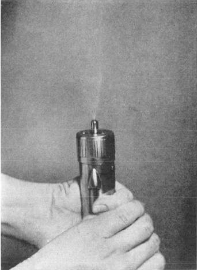
FIG. 6. The terminal phase of the hypospray pattern of spread against air resistance.
