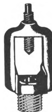
Figure 6-4. Yoke adapter for connecting oxygen regulator to size D cylinder.
